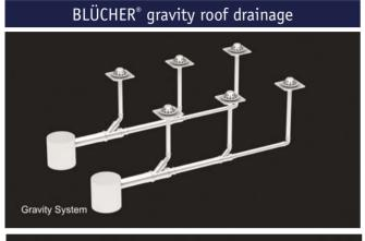
Traditional gravity system with drains spread over the roof area and water led from the roof through downpipes to a belowground pipework system
