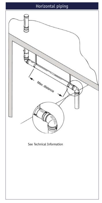
One fixing point per storey is normally sufficient. As opposed to plastic pipes, stainless steel pipes require only one pipe hanger per 3 metres, resulting in less sound and faster installation.
