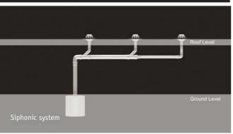
Siphonic system with fewer drains and a small-diameter horizontal pipework system underneath the ceiling. More water is transported through the pipework due to faster flow and a filled pipework system, reducing if not completely removing below-ground drainage.
