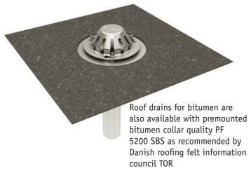
In connection with single ply roof membranes it is important that the sealing material of the roof drain matches the material of the membrane to avoid migrating of softeners from PVC to the other material, since this could make the PVC material brittle, resulting in a higher risk of cracking.
