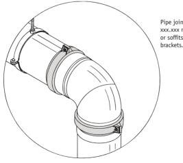
Pipe joint clamps type no. 847. xxx.xxx may be required if walls or soffits are not accessible for
