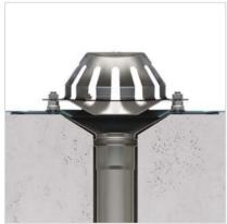
Owing to the siphonic plate of the drain, the pipe is quickly 100% filled, keeping air out of the system and allowing full bore discharge to induce a siphonic action resulting in higher velocities and greater discharge.
